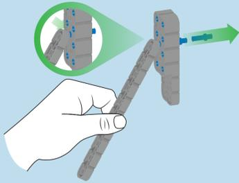
Quickly remove Connector Pins by pressing a VEX IQ Beam against the back of the Pin and pulling it out.
