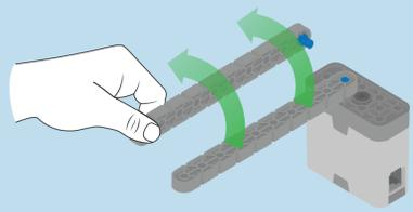
Standoffs and Standoff Connectors can be separated by pressing a shaft through the Standoff Connector.
