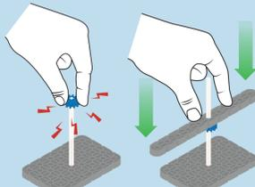
Use a 1x Beam for extra leverage when mounting small VEX IQ elements on shafts.
